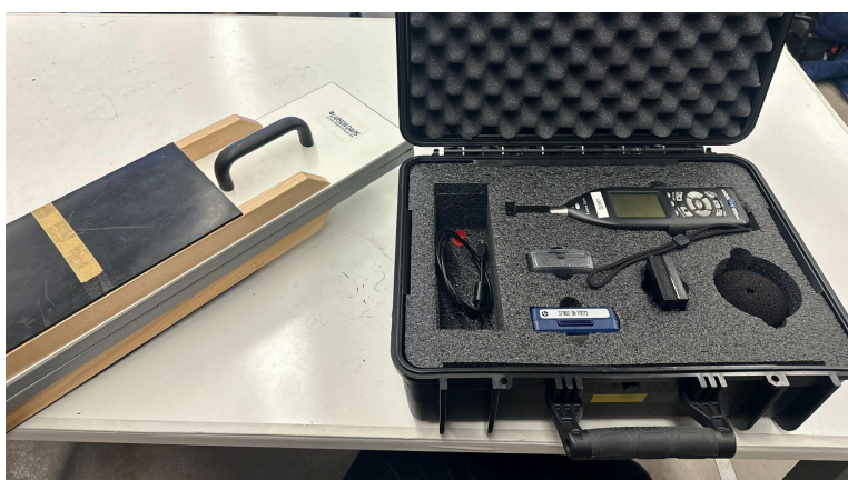
Figure 3: Clapper and SLM Model 831 for Data Acquisition
