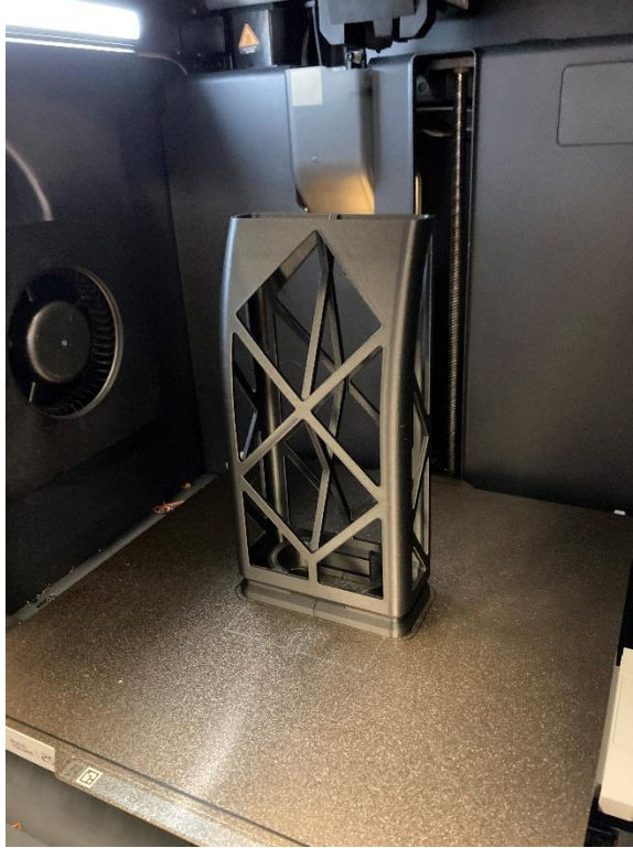
Figure 3: PETG cage after printing. The design uses no support and requires no cleanup.
