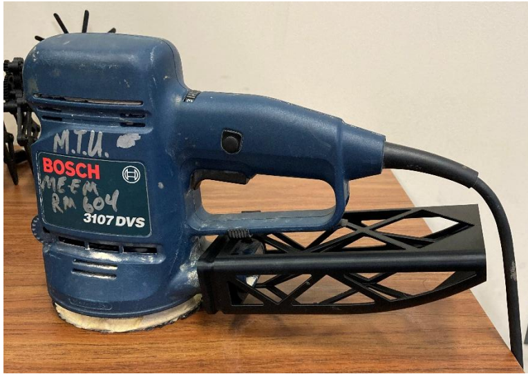
Figure 5: Cage self-secured onto dust port. The dust bag is currently removed.
