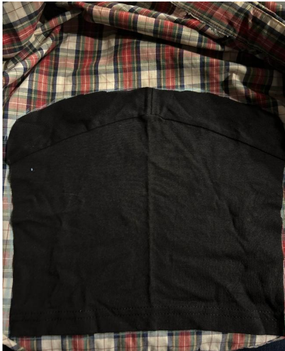
Figure 4: 1st and 2nd layer of dust bag. The 1st cotton layer has been fitted to the cage and is now being traced onto the next layer.
